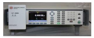
Figure 3-7: SCA -8588A on the Fluke 8588A
