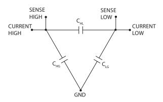
*Figure 3-5: SCA as a 5-terminal capacitor To use as a 2-terminal capacitor, connect to only the two SENSE terminals.*
