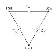
Figure 3-2: Capacitance shunted by leakage to case
